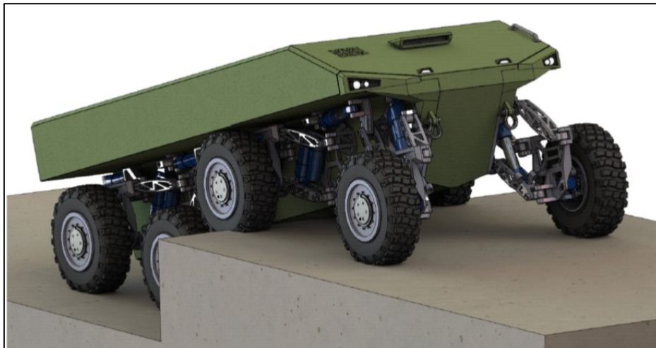
Figure 2: Advanced long travel active suspension system concept (Courtesy QinetiQ)
